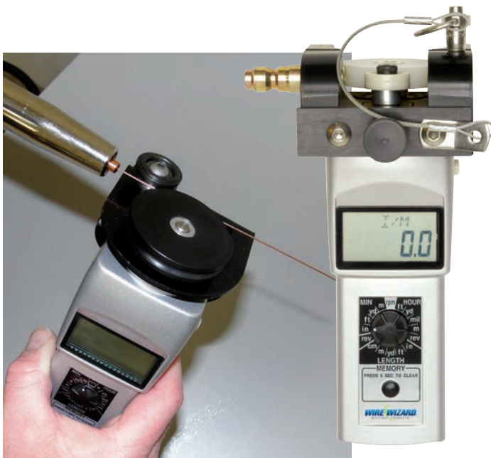
HHSS-12 obtaining measurement at the torch end
