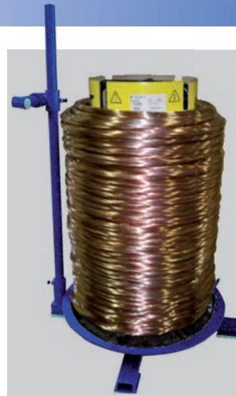
WWTT-1000: Length x Width: 100x100 cm Weight : 192 Kg Max. Load : 1.000 Kg
