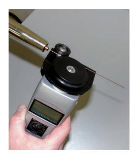
HHSS-12 obtaining measurement at the torch end
