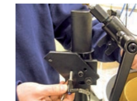
Removable guide arm for easy drum change
